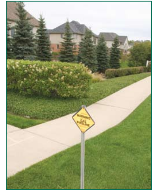
Markers identify nearby pipelines.
