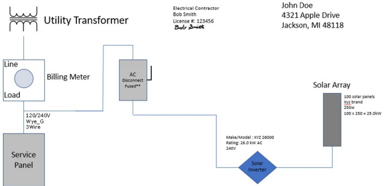
The Total Generator Nameplate AC Rating (kW): Is calculated by the number of inverters multiplied by the inverter power rating (kW\_AC) per inverter.
