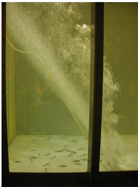
Figure 4-2 Air Bubble Curtain (Courtesy of Alden)
