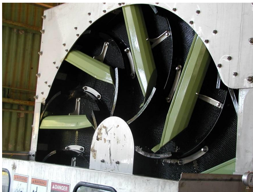
Figure 4-8 Bilfinger Multi-Disc Screen with Fish Lifting Buckets (Courtesy of Bilfinger)
