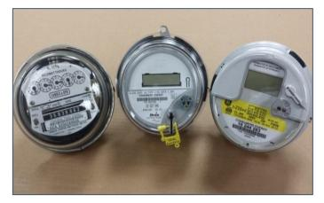
Three types of meters are commonly used to measure electricity: electromechanical meters (analogue technology – similar to analogue clocks), digital technology meters, and digital meters with communication capabilities -- also known as smart meters.
