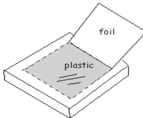
3. Be sure the plastic becomes a tightly sealed window so air cannot escape from the oven interior.
