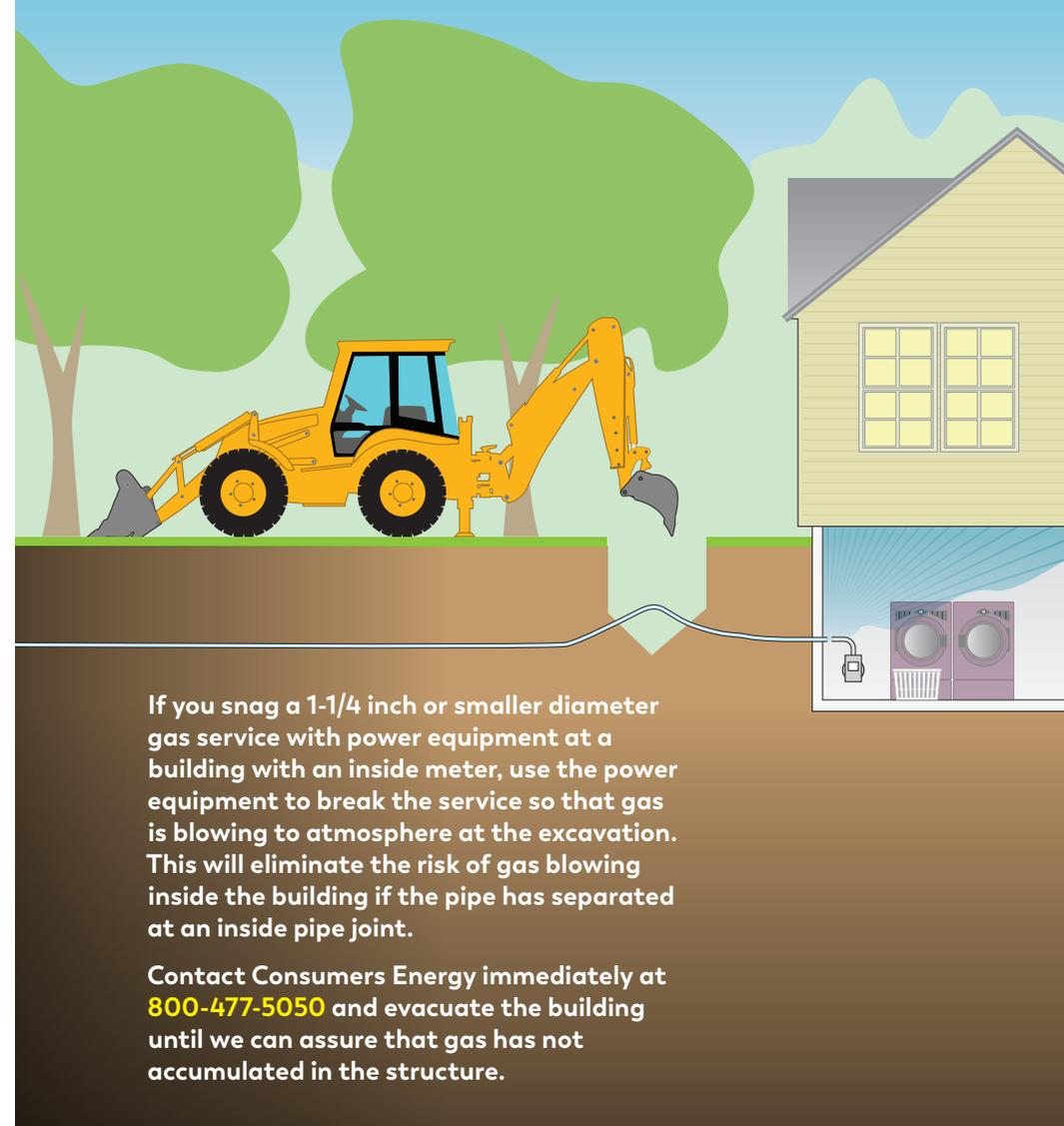
**If you snag a 1-1/4 inch or smaller diameter gas service with power equipment at a building with an inside meter, use the power equipment to break the service so that gas is blowing to atmosphere at the excavation. This will eliminate the risk of gas blowing inside the building if the pipe has separated at an inside pipe joint.**
