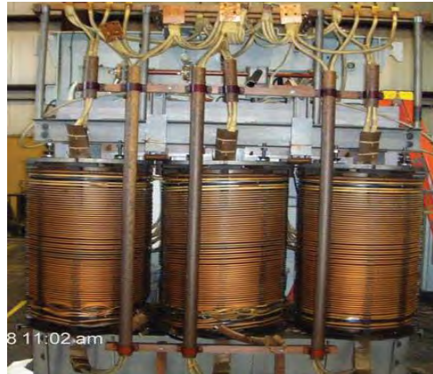
FIGURE 59 – AC TRANSFORMER FAILURE AT GLADWIN SUBSTATION
