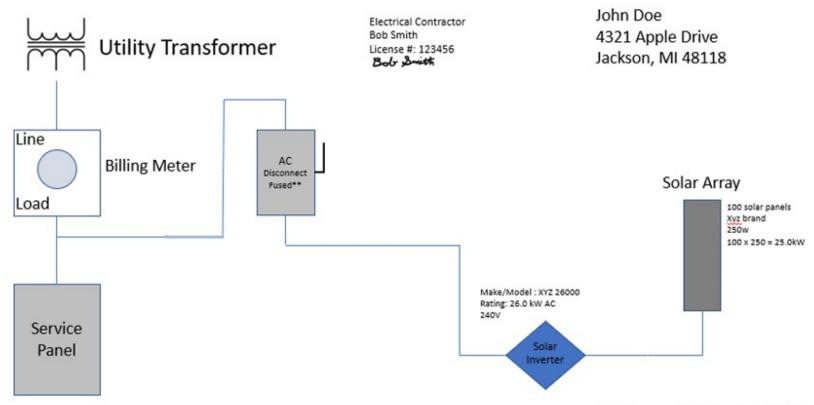
AC disconnect to be located within 5' of meter
