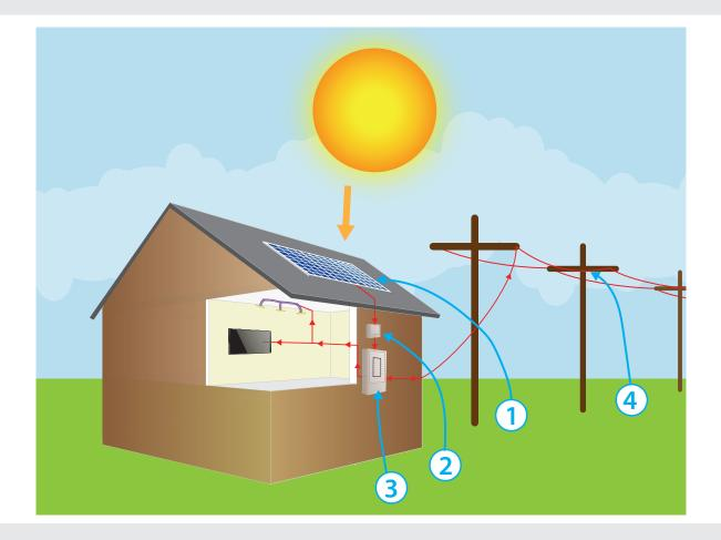
**SOLAR PHOTOVOLTAIC PANELS:** Produce DC (direct current) electricity when photons of light from the sun strike the panel's surface
