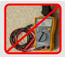
**Voltage testers** – NOT to be used to test downed wires! Only use voltage testers for household current testing (inside the house, plugs, etc).
