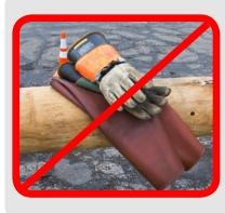
**Rubber gloves** – NOT to be used for moving wires! The rubber gloves that are used by Consumers Energy employees are tested regularly, specifically approved for working on our electric facilities and are designed to protect against electrocution.
