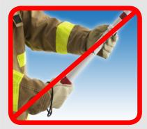
**Hot sticks** – NOT to be used for moving wires! Hot sticks are used only to alert you if a vehicle or another object is energized. Make sure your tools are up to date and calibrated frequently. They are also shock sensitive.
