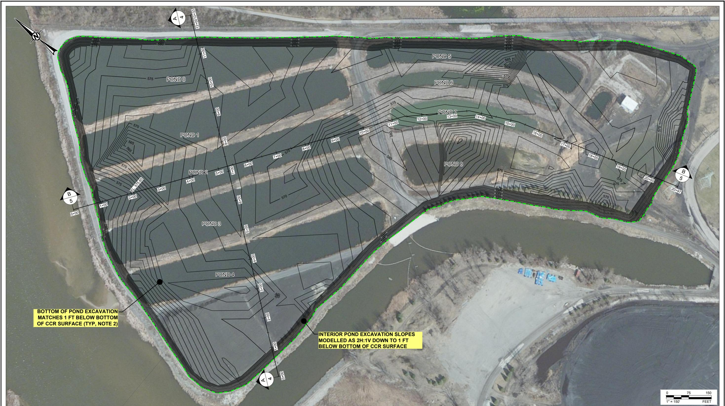
**BOTTOM OF POND EXCAVATION MATCHES 1 FT BELOW BOTTOM OF CCR SURFACE (TYP, NOTE 2)**
