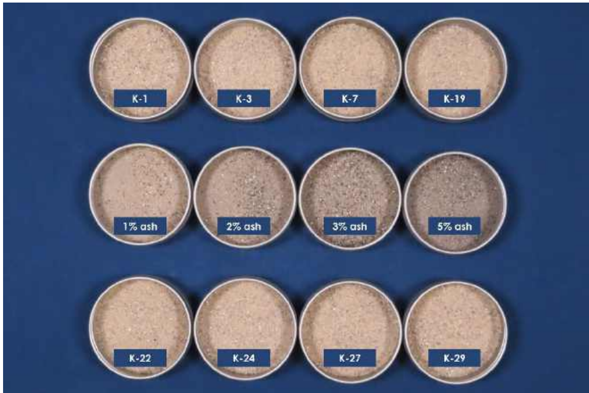
Figure 9 – Comparison of processed 2NS sand type samples to select reference standards (middle row).
