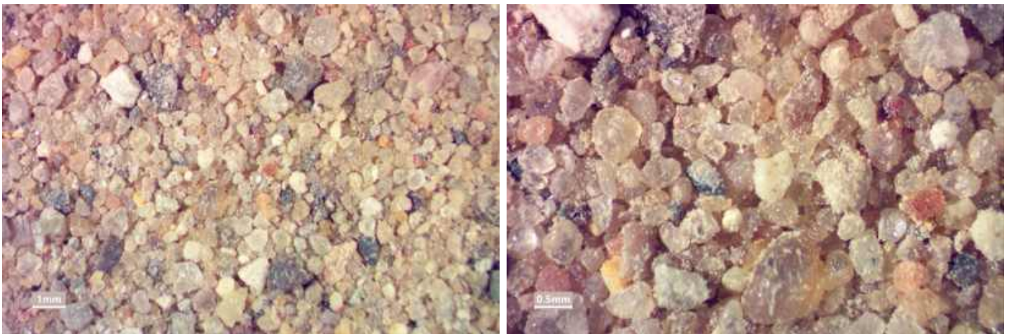
Figure 12 – Magnified views of processed sample K-24, also representative of 2NS sand type.
