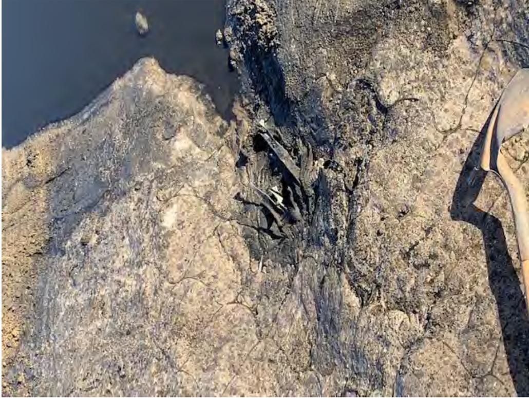
*Figure 1 - Visual Identification of Primary Liner Damage – Shovel on the Right for Scale*
