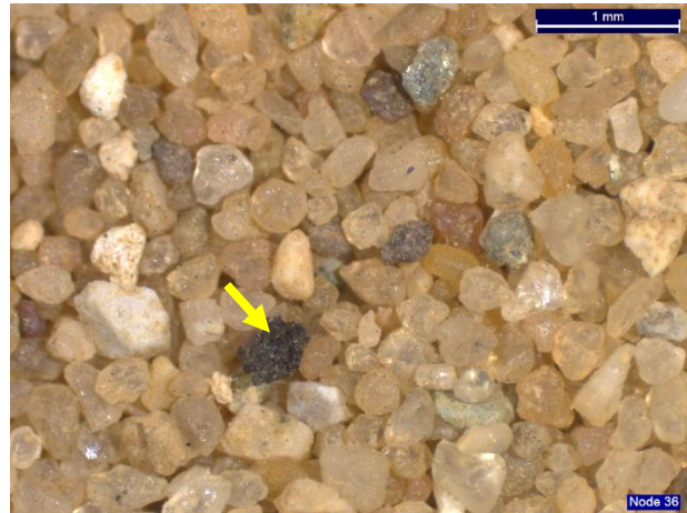
The sample is clean sand that mainly consists of white, pale yellow, and colorless transparent quartz. Dark red, green, brown, and gray particles of various minerals and rocks are common. Arrow shows a CCR particle.
