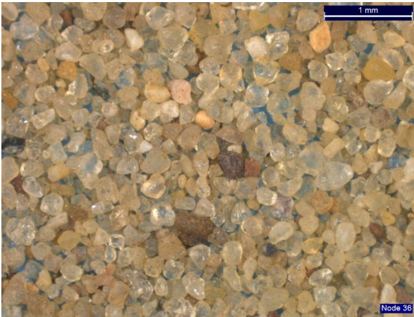
The sample is clean sand that mainly consists of white, pale yellow, and colorless transparent quartz. Dark red, green, brown, and gray particles of various minerals and rocks are common. Arrow shows a CCR particle.
