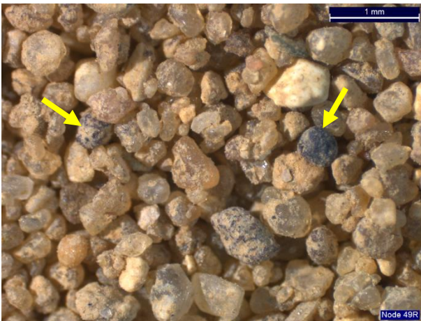
Arrows show spherical black CCR particles that are partially coated with silty material.
