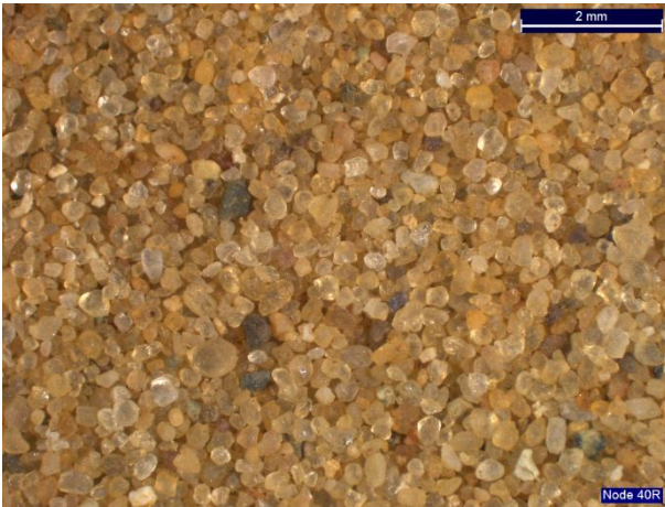
The sand is unevenly coated with yellow silty material. Darker colored particles are mostly schist, chert, and granite.
