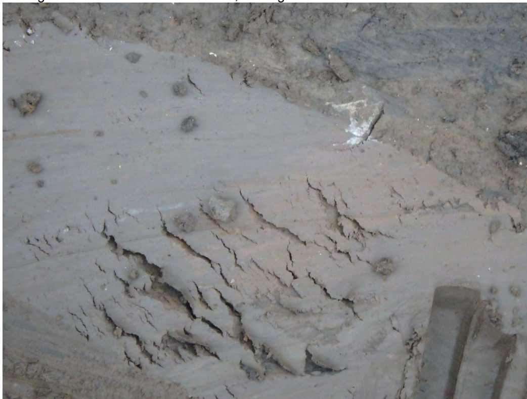
Clean clay on floor of Chemical Pond B left after removal of residual.
