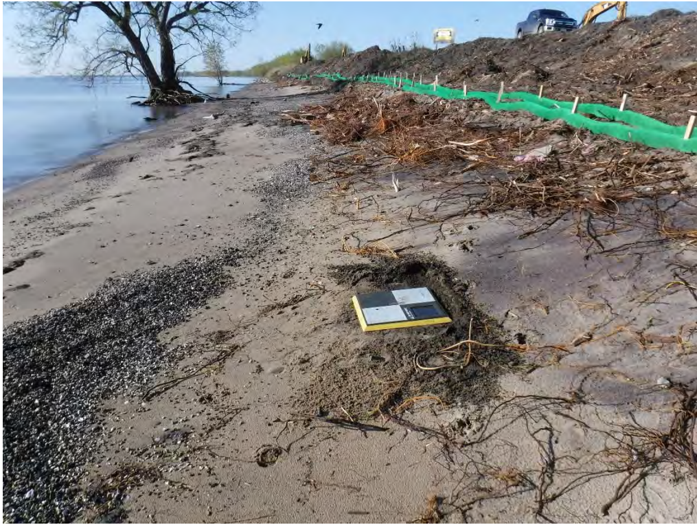
Control set for existing conditions drone survey.
