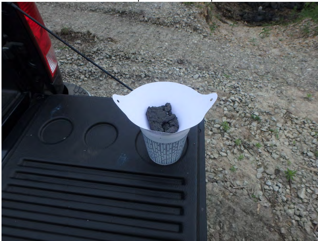
Paint Filter test of residual material from Chemical Pond A
