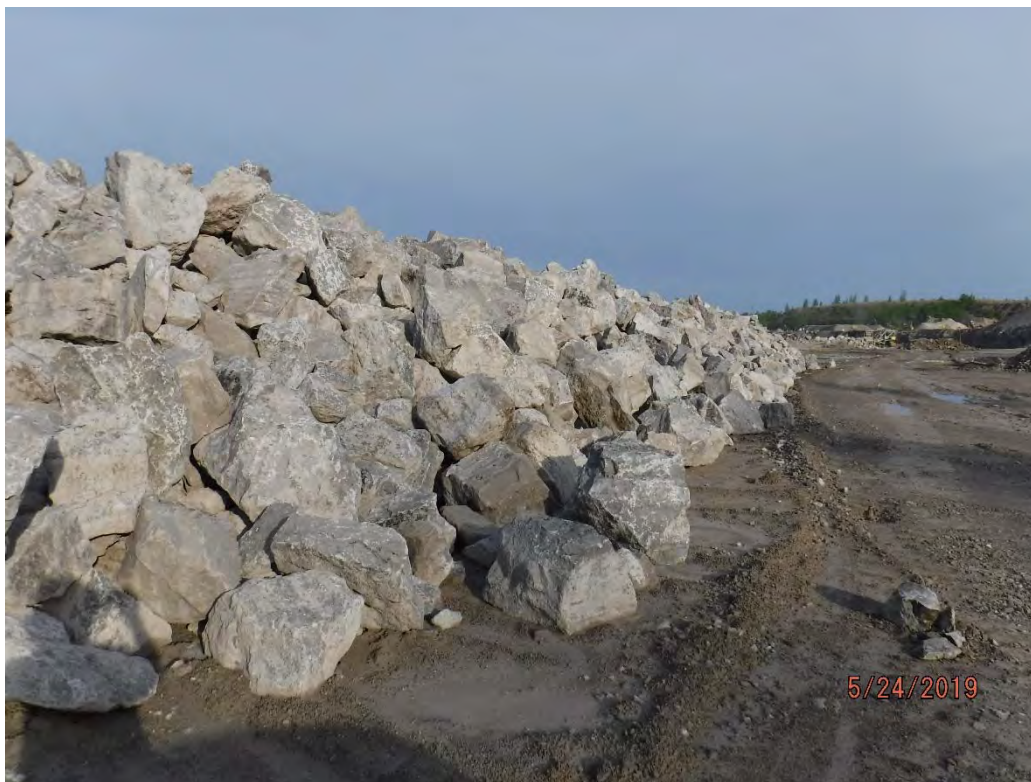
Onsite at Aggregate Industries inspection large riprap proposed for shoreline protection.
