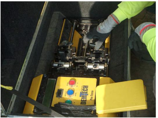
Testing of trial weld prior to start of seaming.
