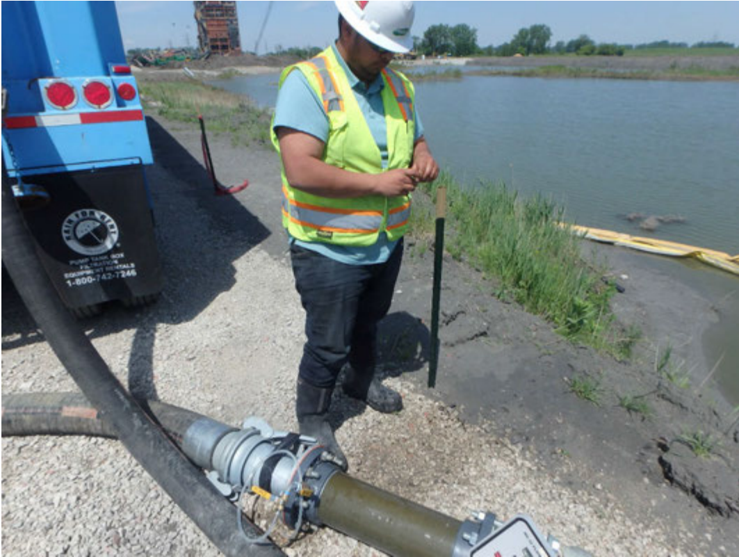
ProAct performing turbidity test on water being pumped from Pond 2.
