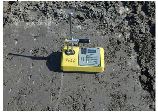
Density testing of compacted structural fill in Pond 1.
