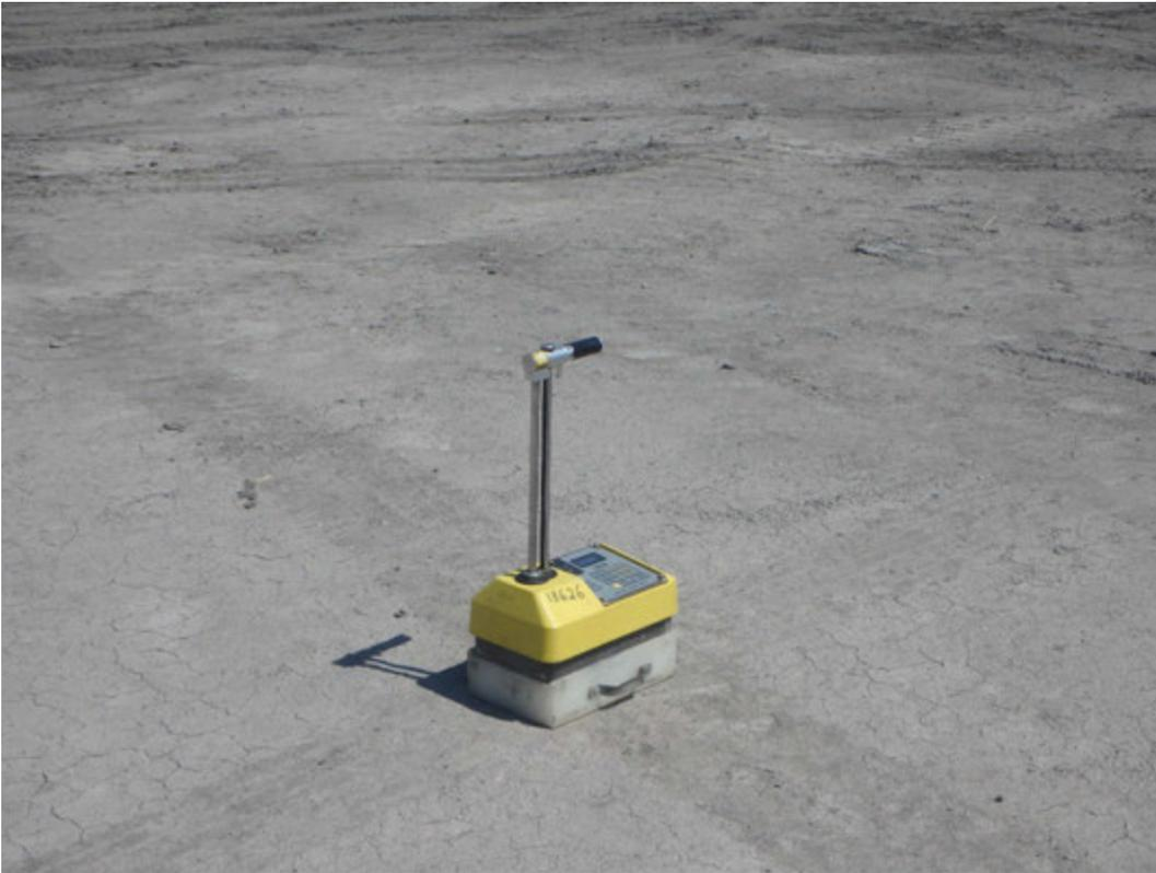
Performing Standard Test prior to start of density testing.
