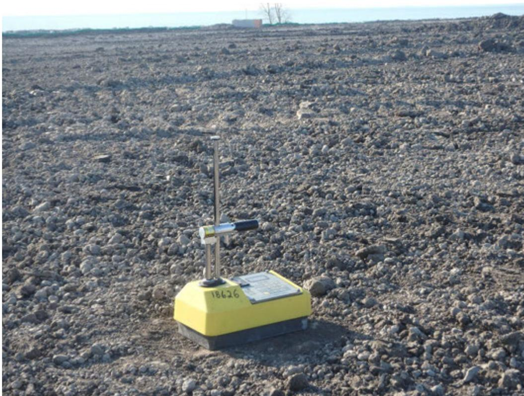
Density testing structural fill lift in Pond 2, looking east.
