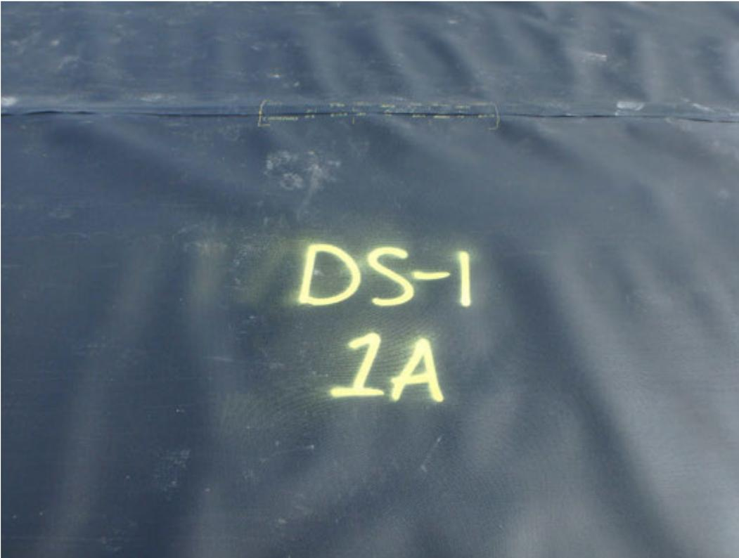
Destruct location marked for removal and testing.
