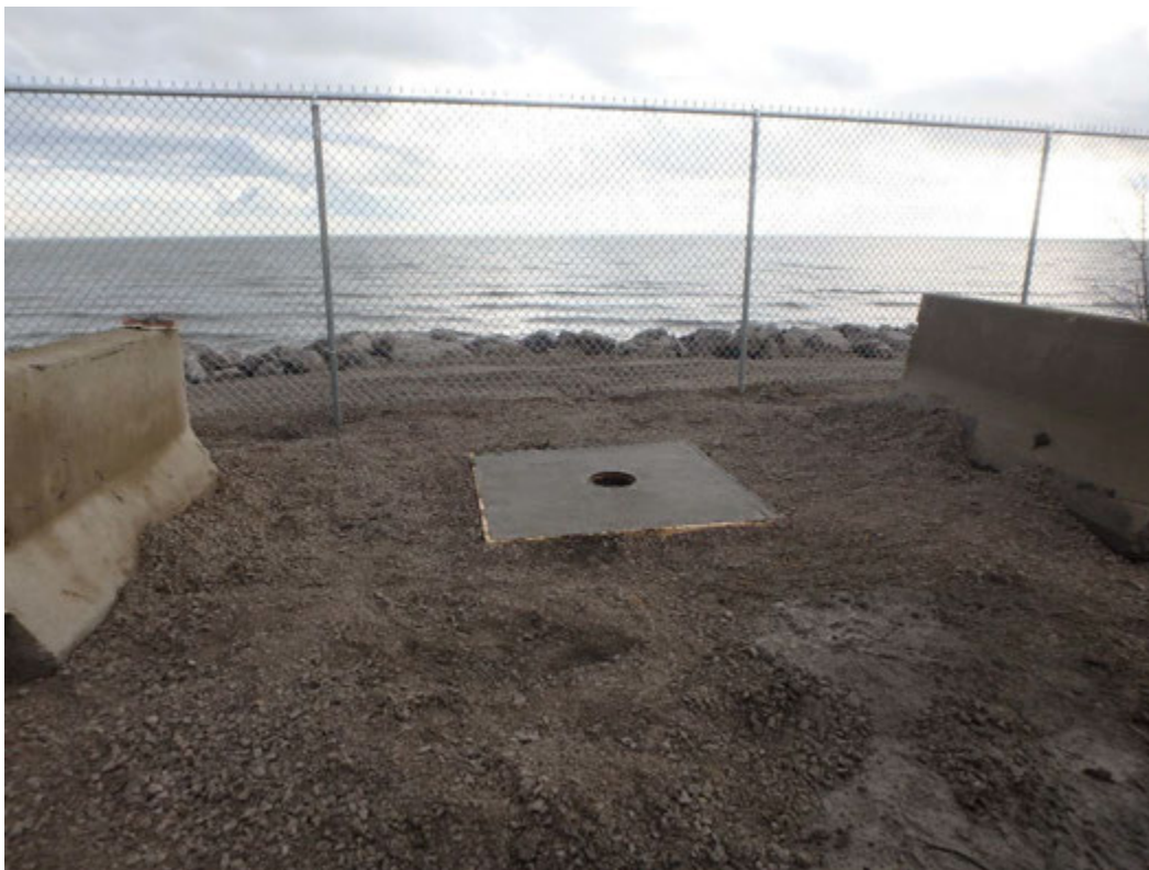
MW-15003 ground flush in east access road
