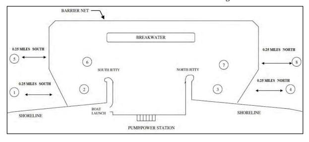
Figure E-4.3.3-2: Gill net sampling stations (numbered circles) used for barrier net effectiveness monitoring.
