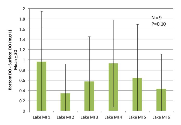
Figure 7. Mean and Standard Deviation of Bottom Dissolved Oxygen Minus Surface Dissolved Oxygen for Six Lake Michigan Sampling Sites.
